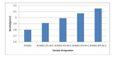
Figure 1 Variation of density of Al 6061 alloy and Al6061-nickel coated composites
