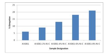
Figure 3 Variation of ductility (%age elongation) of Al 6061 matrix alloy and the developed nickel coated cenosphere composites
